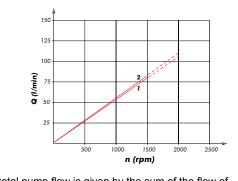
The total pump flow is given by the sum of the flow of each pressure port.
