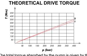
The total torque absorbed by the pump is given by the sum of the torques necessary to give pressure to the pressure ports.
