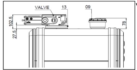
Valve mounted on top of tank
