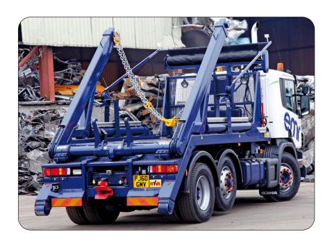
The steel platform is provided with two wearing strips in longitudinal direction. 6 adjustable container stops can be located through side steaks in the platform.
