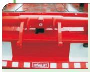
One tipping chain, length 650mm with open safety hook is mounted on the torsion tube. A second tipping chain or tipping hooks are available as an option.
