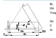
body length rear overhang vert. pos. centre of gravity pivot length bracket length tipping angle stroke x 60 / Qo
