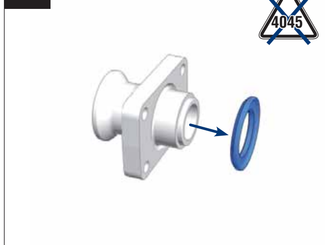
Demontage der Lagerbuchsen / Stangenführung (1) Dismantling of bearing bushing / rod guidance system (1)
