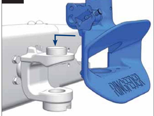
Montage des Kuppelkörpers Fitting of the coupling assembly
