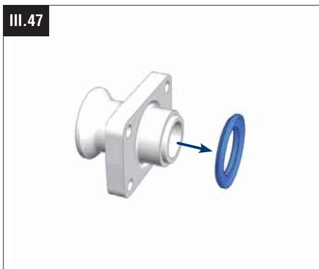
Demontage der Lagerbuchsen/Stangenführung (1) Dismantling of bearing bushing/rod guidance system (1)
